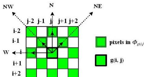
Fig 4: Four possible directions associated with green pixel
