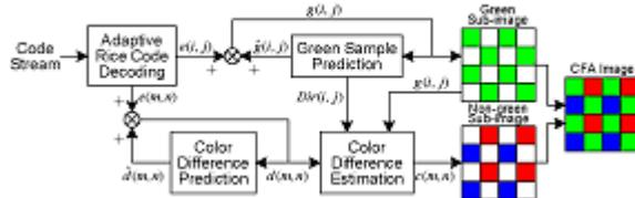
Fig 5: Structure of Decoder
