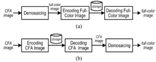
Fig 2: single sensor camera imaging chain (a) demosaicing and
