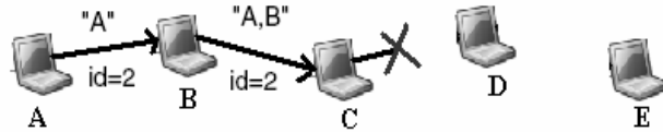
Fig.2: Node C is unable to forward a packet from A to E over its link to next hop D.
