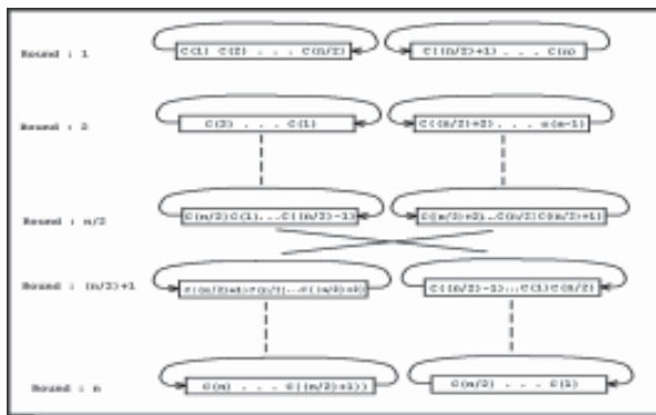
Figure (9): The relationship between Round number and the Column orders of S-Box
