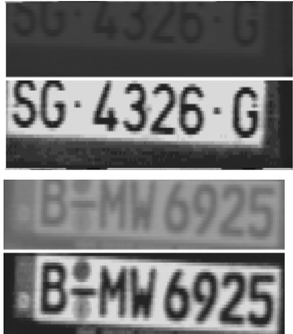
Fig 3: Number plate Recognition before & after Histogram process
