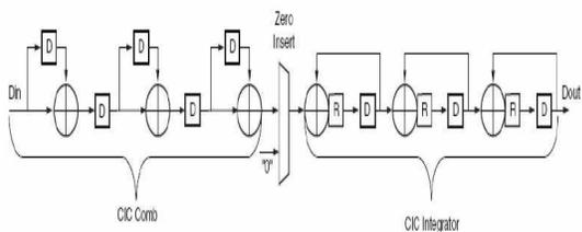
Figure 2. CIC Filter Structure Block Diagram
