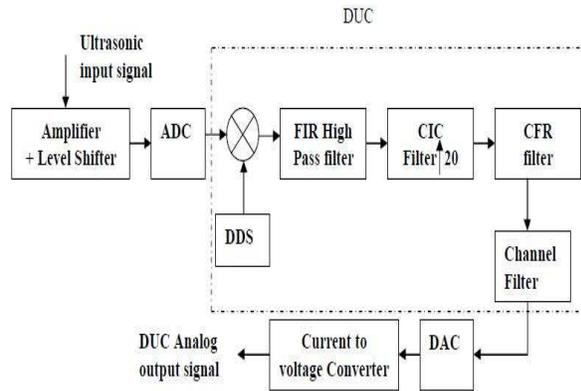
Figure 1. Digital Up Converter Block Diagram
