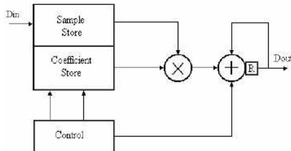
Figure 7. Simplified Block diagram of MAC
