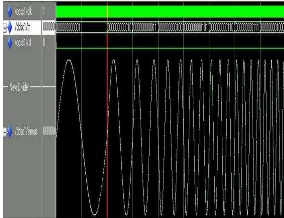
Figure 9. Simulation Results of DDS in MODELSIM
