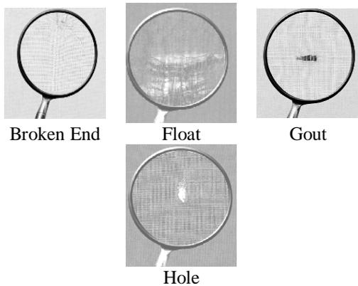
**Figure 2 Weaving defects**
