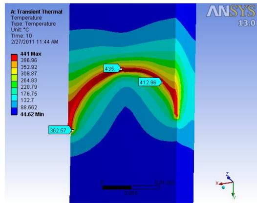
Figure 5. 3D transient temperature mapping of workpiece
