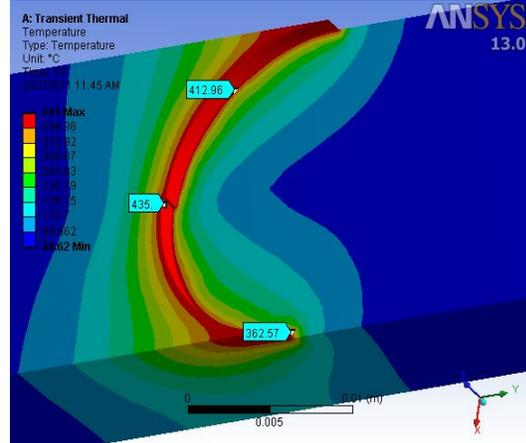
Figure 4. 3D transient temperature modeling of cutting zone
