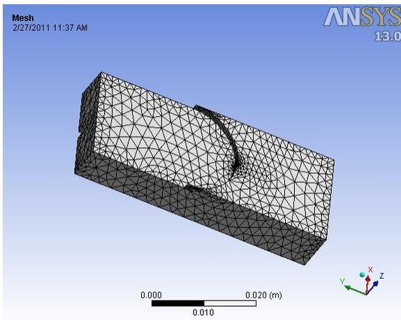
Figure 3. Workpiece after 3D tetrahedral mesh generation
