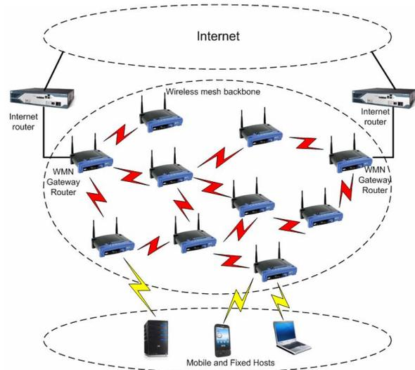
**Figure 1: Wireless Mesh Network (WMN) Architecture**
