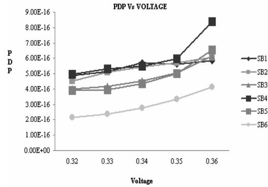
**Fig. 12 Power-Delay Product at different voltages in 65 nm technology**
