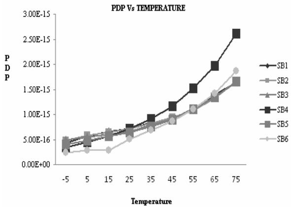
**Fig. 9 Power-Delay Product Vs temperature at 45 nm technology**
