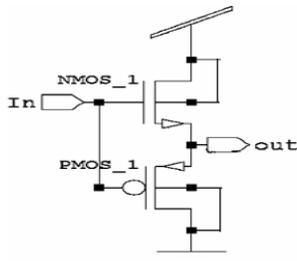
**Fig. 1 conventional body-biasing inverter**
