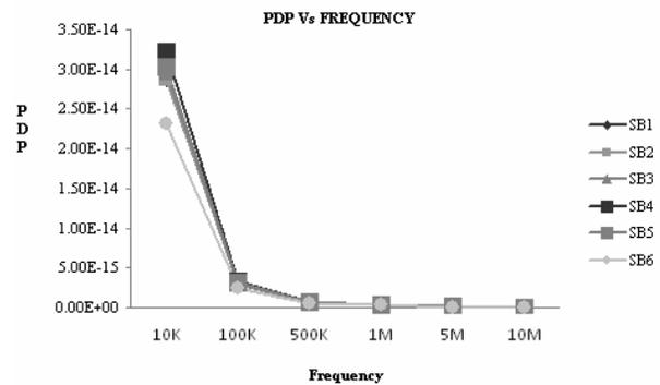
Fig. 6 Power-Delay Product Vs frequency in 45 nm technology
