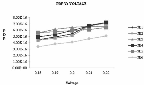
Fig. 4 Power-Delay Product at various voltages in 45 nm technology
