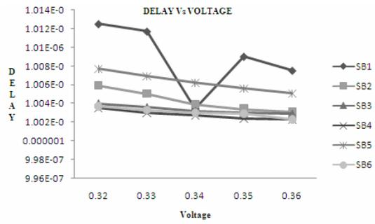
**Fig. 11 Delay at different voltages in 65 nm technology**
