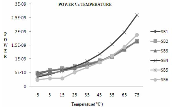
Fig. 7 Power Consumption Vs temperature at 45 nm technology
