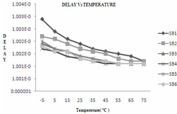
**Fig. 8 Delay at various temperatures in 45 nm technology**
