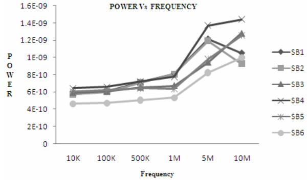
Fig. 5 Power Consumption at different frequencies in 45 nm technology
