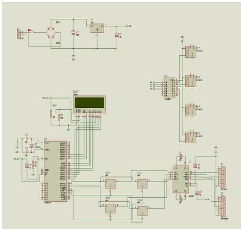
Figure 2. Circuit design for vehicle locking and tracking system using PROTEUS software
