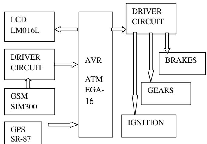
Figure 1. Block schematic for vehicle locking and tracking system.
