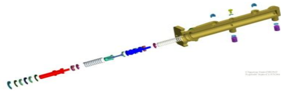
Figure. 6 Exploded View of the master Cylinder
