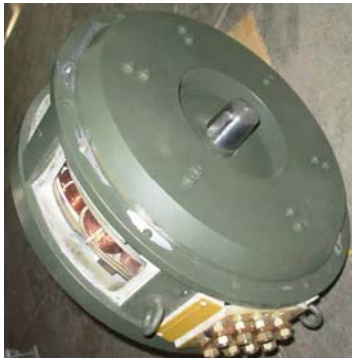
Fig.4 Pictorial View of AFPM alternator
