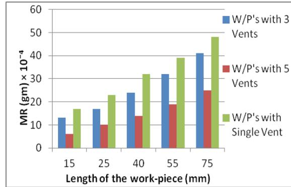
**Fig.5. MR in micromachining work-pieces of varying lengths having different vent considerations**
