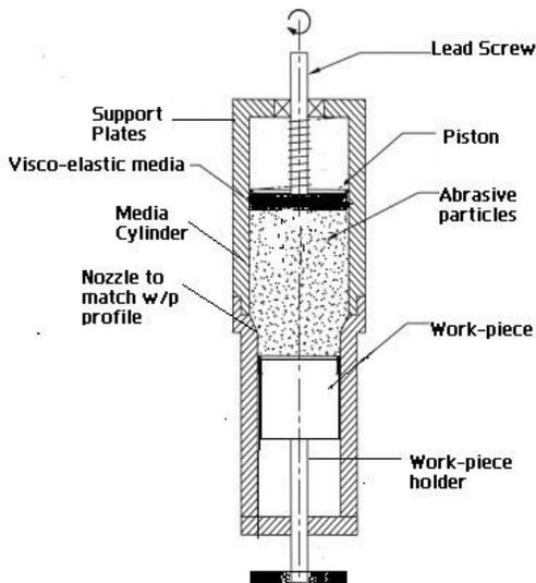
**Fig.1 Assembly drawing of the table-top setup for an AFM process**
