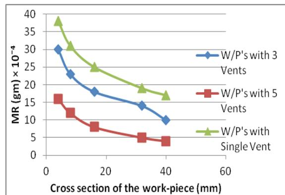
**Fig.2. Effect of different vent considerations in work-pieces of varying cross sections on MR**
