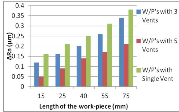
**Fig.9. ΔRa in micromachining work-pieces of varying lengths having different vent considerations**
