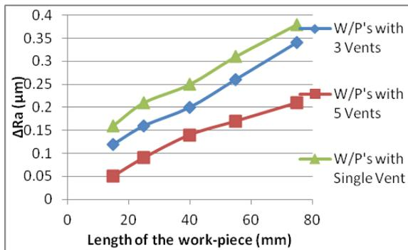
**Fig.8. Effect of different vent considerations in work-pieces of varying lengths on ΔRa**
