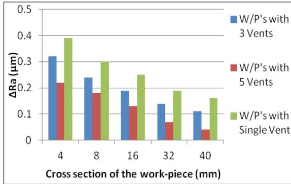
**Fig.7. ΔRa in micromachining work-pieces of varying cross sections having different vent considerations**
