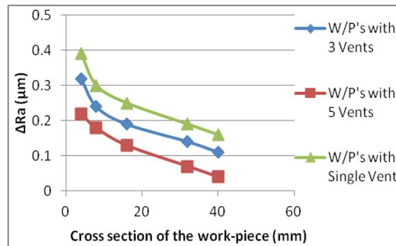
**Fig.6. Effect of different vent considerations in work-pieces of varying cross sections on ΔRa**
