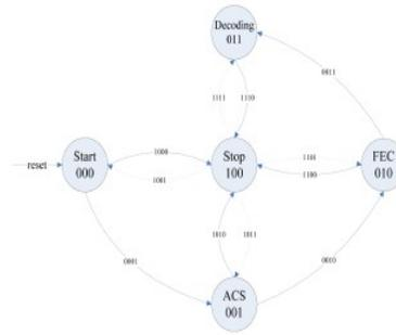
Fig.4 The Finite State Machine of Viterbi decoder
