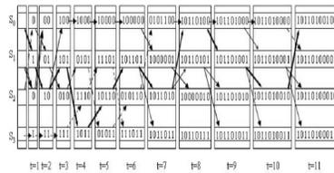
Fig.3 Register Exchange (RE) Method
