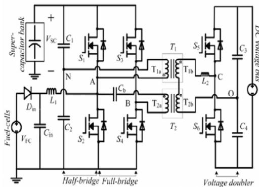
**Figure. 2. The proposed hybrid bidirectional DC-DC converter topology.**
