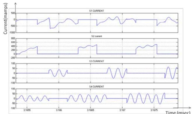
**Figure. 8. Switching currents of boost mode of operation**
