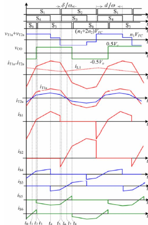
**Figure. 3. Timing diagram and typical waveforms in the boost mode.**
