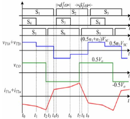
**Figure.6. Timing diagram and typical waveforms under the super capacitor researching mode**
