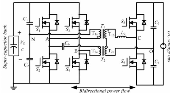
Figure. 4. Converter topology in capacitor power mode
