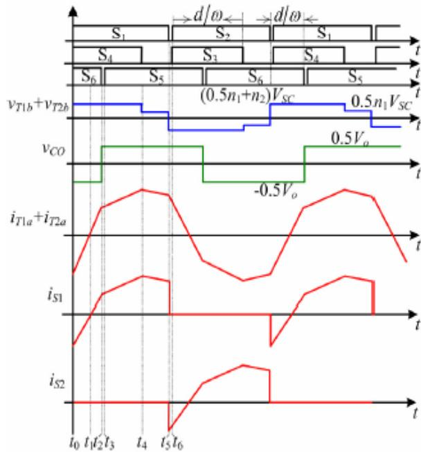
Figure.5. Timing diagram and typical waveforms under the super capacitor power mode
