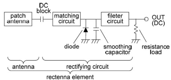
**Figure .4. Block diagram of the Rectenna Element**
