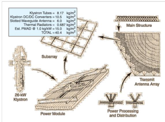
Figure.2. Klystron transmitter
