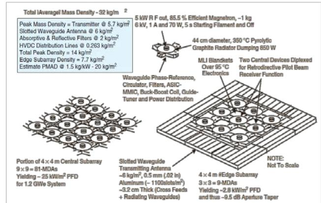
Figure.3. Magnetron directional amplifier transmitter
