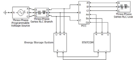
Figure 1. Schematic representation of the FD-STATCOM
