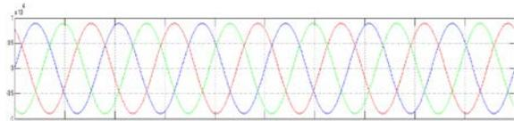
**Figure.9. Load voltages with FD Statcom under LL Fault**
