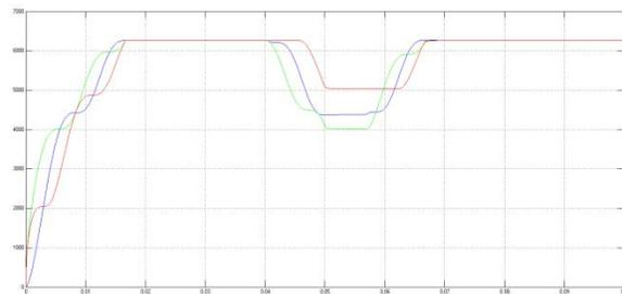
**Figure. 6. RMS voltages without FD Statcom under LL Fault**
