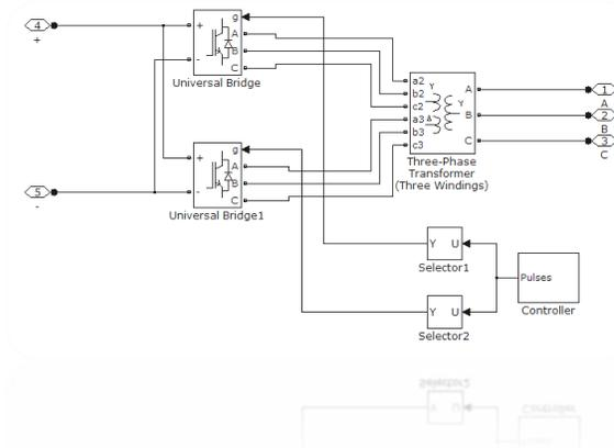
Figure 2. The 12-pulse FD-STATCOM arrangement
