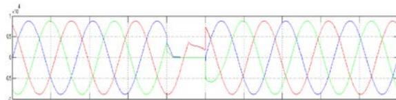
**Figure. 12. Load voltages without FD Statcom under DLG Fault**
