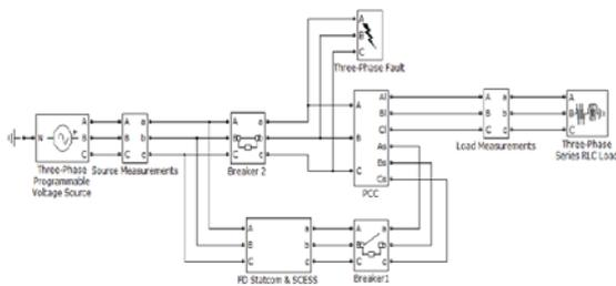
**Figure. 5 shows the test system implemented in MATLAB/SIMULINK to carry out simulations for the FDSTATCOM.**
