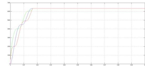
**Figure. 13. RMS voltages with FD Statcom under DLG Fault**
