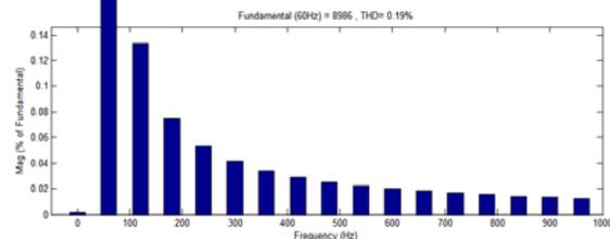
**Figure. 18. Frequency Spectrum of load voltages under islanded condition**
