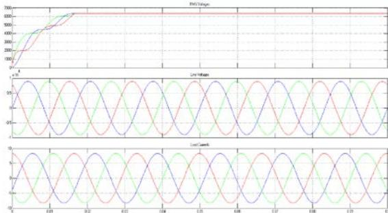
**Figure. 17. PCC Measurements under islanded operated condition with FDStatcom**
