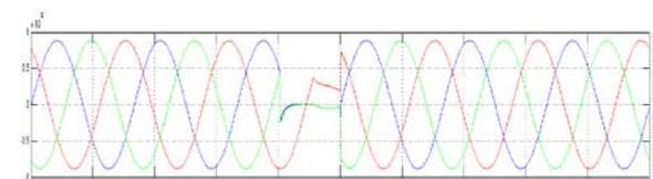
**Figure. 7. Load Voltages without FD Statcom under LL Fault**
