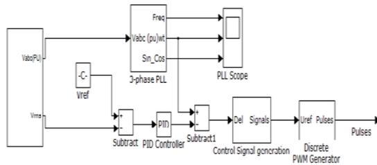
**Figure. 3. Control scheme designed for the FD-STATCOM**
