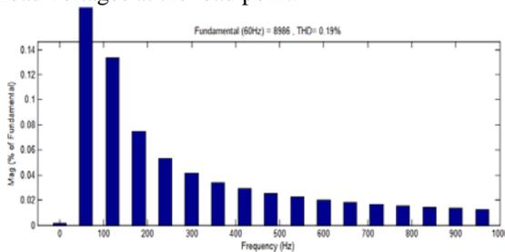
**Figure. 10. Frequency Spectrum of load voltages under LL Fault**
