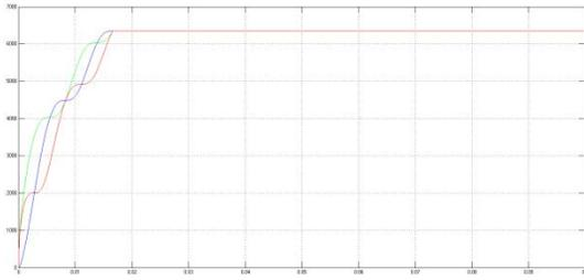
**Figure. 8. RMS voltages with FD Statcom under LL Fault**
