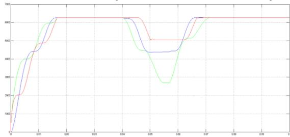
**Figure. 11. RMS voltages without FD Statcom under DLG Fault**
