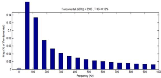
**Figure. 15. Frequency Spectrum of load voltages under DLG fault**
