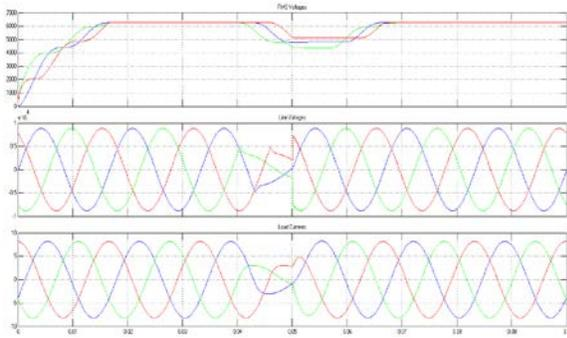
**Figure. 16. PCC Measurements under islanded operated condition without FDStatcom**
