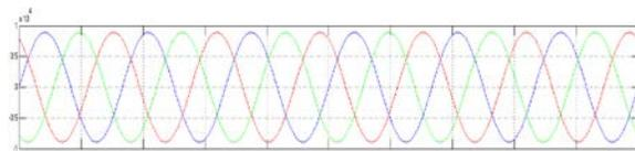
**Figure. 14. Load voltages with FD Statcom under DLG Fault**
