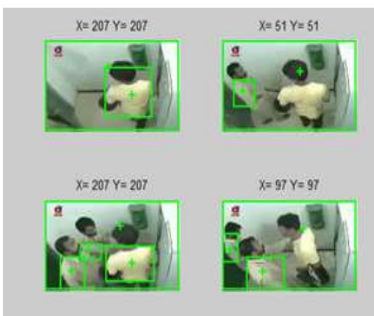
Fig. 7 Centroids of the Bounding Box of the Blobs
