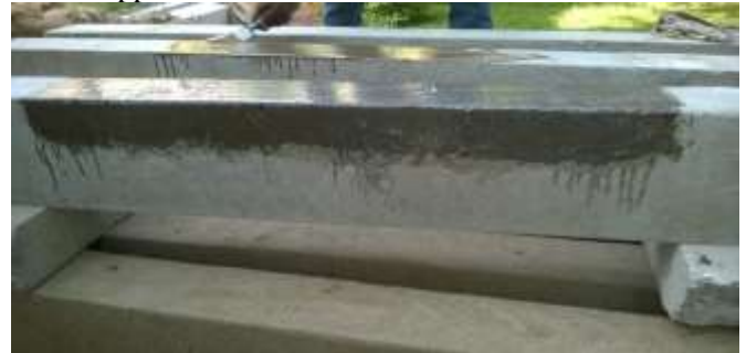
Fig 3.4 Applying primer on beam specimen
