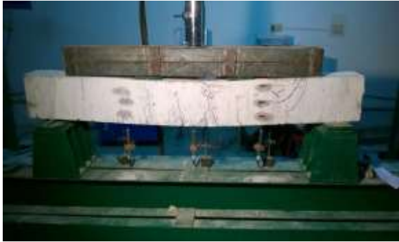
Fig 6.1 Cracking pattern of Control beam
