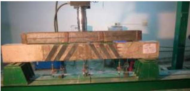
Fig 3.10 Load setup of Inclined Wrap Stirrups
