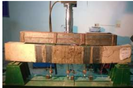
Fig 6.5 Cracking pattern of VWS specimen
